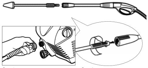
Step 1 Connect the high pressure hose to the unit's high pressure outlet.
